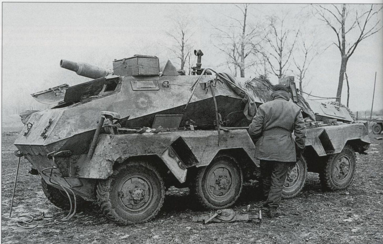
This old veteran, a SdKfz 233 s.Pz.Sp.Wg (7.5cm), was lost in the Celles pocket in late December 1944 in the fighting with the US 2nd Armored Division. The trident insignia on the bow identifies it as belonging to the 2. Panzer Division. This particular family of 8x8 armored cars had largely been superseded in 1944 by the newer SdKfz 234 series, but some old veterans like this one continued to serve until lost in combat.
