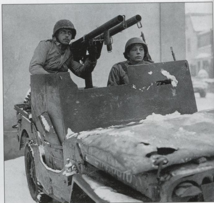
This other view of the bazooka armed jeep from a 60th Infantry I&R platoon also shows how the crew has added a partial armored shield around the front of the vehicle from plate steel.
