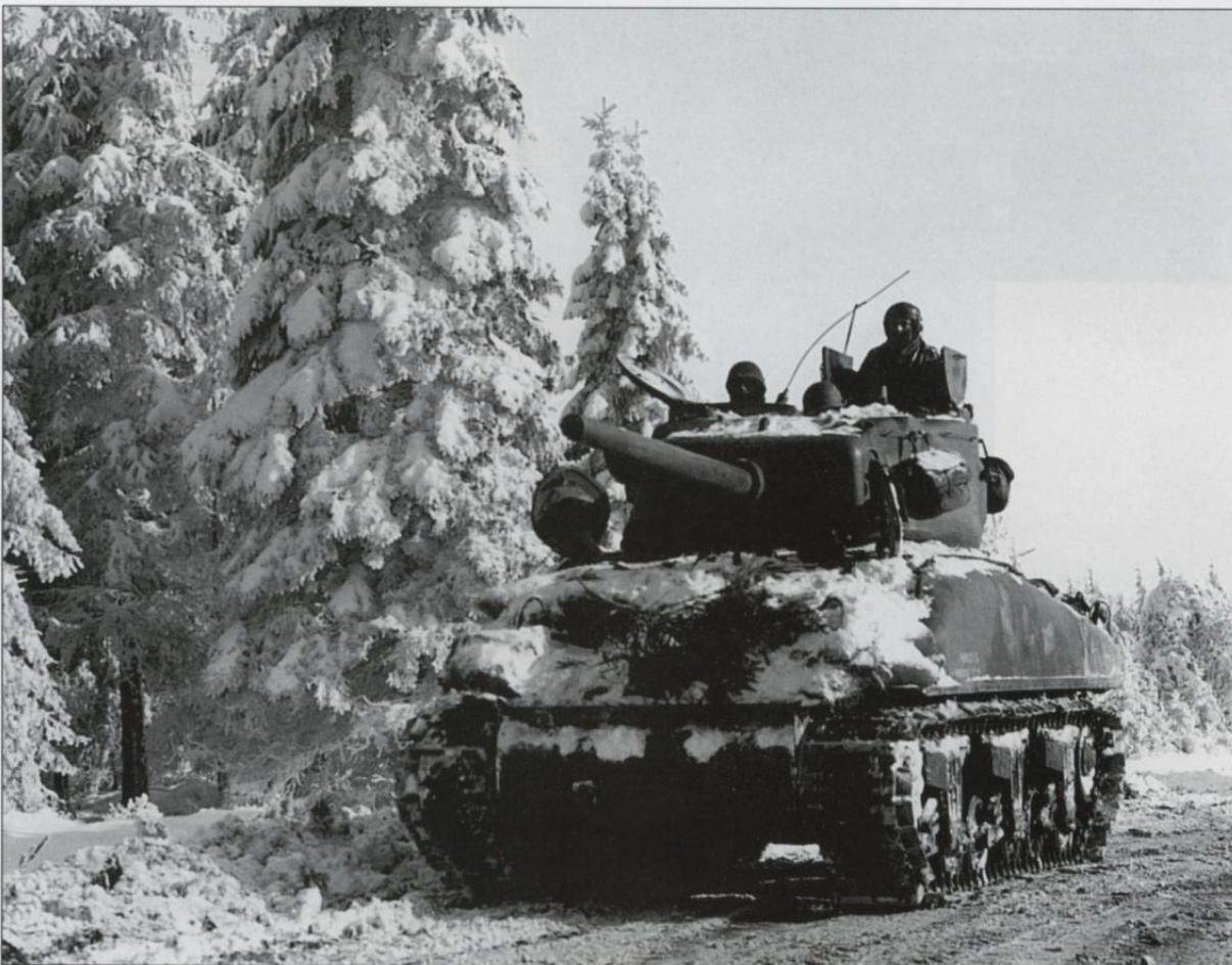
The crew of a M4A1 (76mm) of the 4th Armored Division add foliage to their tank in an effort to improve its camouflage near Kiewelbach, Luxembourg on 18 January 1945. This tank is fitted with metal chevron track and duck bill end extenders.
