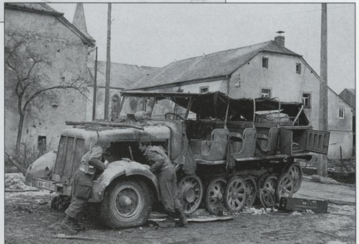
A Daimler-Benz DB 10 12-ton Zugkraftwagen of 2. Panzer Division lies disabled in the streets of Marnach, Luxembourg following the recapture of the town by the 26th Infantry Division on 25 January 1945. This vehicle was used in panzer divisions to tow heavy artillery.
