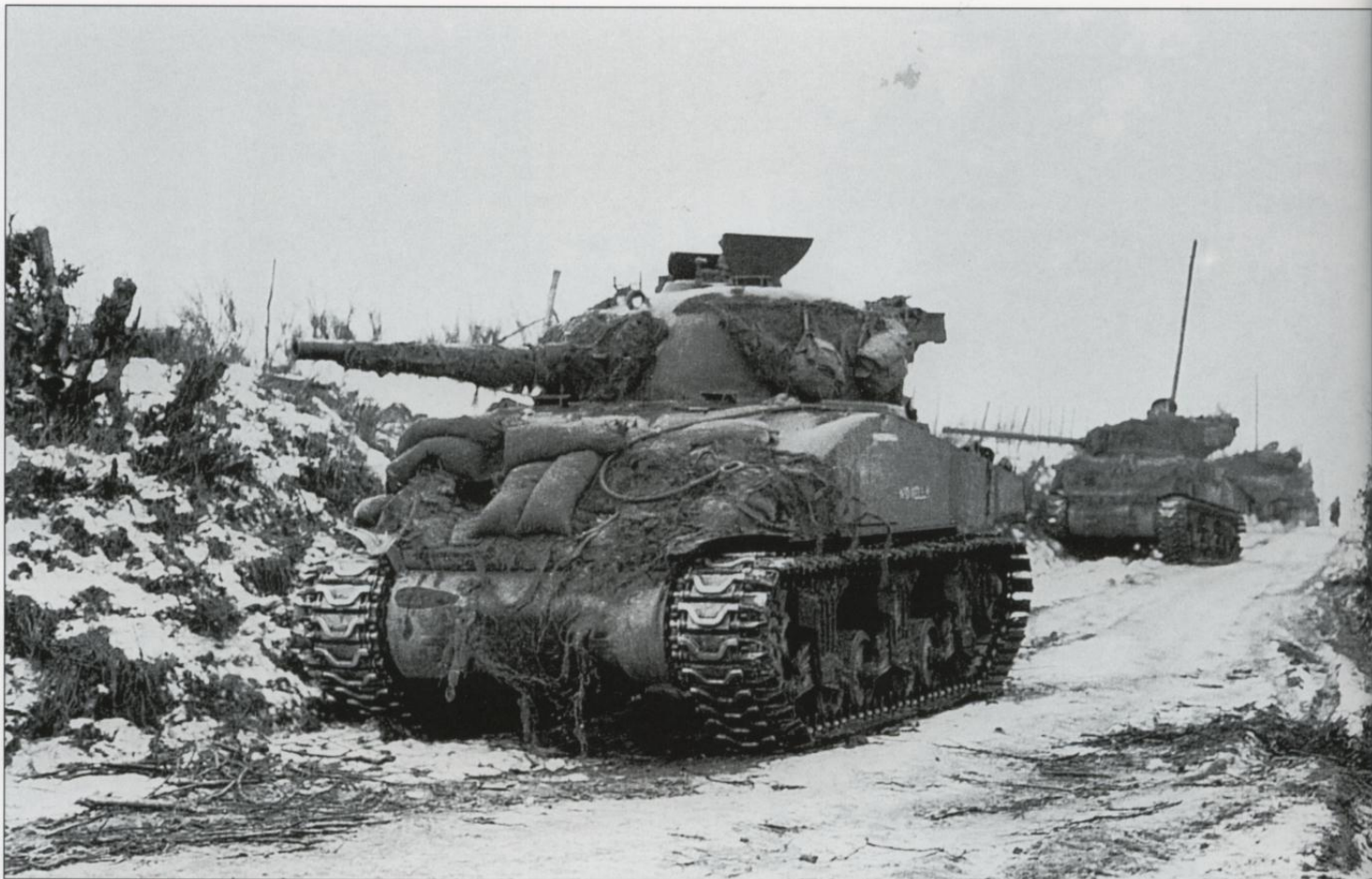
Tanks of the 2nd Armored Division support the 84th Division during the fighting near Amonines, Belgium on 2 January 1945. The lead tank appears to be a composite hull M4. It is fitted with the T54 metal chevron tracks with duck bill extenders. There was quite a bit of variation in the detail of the duck bills, as many were manufactured locally in shops in Belgium and France.
