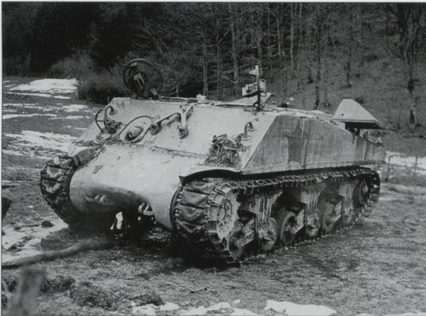
German units made use of captured equipment when possible, especially the German Seventh Army which was short of tanks. This M4A3 medium tank was knocked out by the 10th Armored Division at the end of January 1945 during the fighting in Luxembourg, losing its turret. The US white stars on the side had been painted out, and barely evident on the bow is a German cross.
