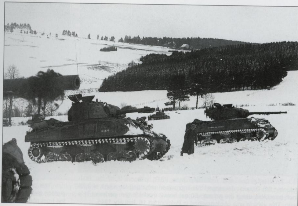
A M4A3 (76mm) of the 750th Tank Battalion moves into Salmchateau in support of the 75th Division on 16 January 1945. The tank has been thoroughly whitewashed, and on the back deck is a long fluorescent orange air identity panel to prevent strafing by Allied aircraft.
