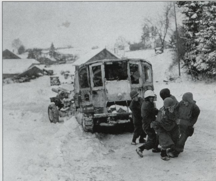
Sometimes even the most powerful vehicle needs a good tug. The crew of this M4 high speed tractor towing a 155mm howitzer is extending the tow cable from the front winch to an unseen vehicle in the foreground to help extract it from a deep patch of snow or ice. This vehicle belonged to the 809th Field Artillery Battalion and is seen near Nederscheid, Belgium on 30 January 1945.
