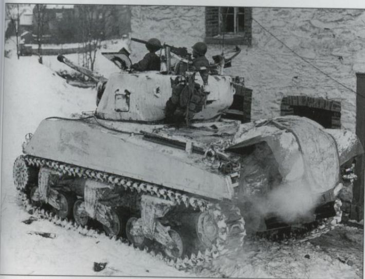
A M4A3 (76mm) of the 750th Tank Battalion moves into Salmchateau in support of the 75th Division on 16 January 1945. The tank has been thoroughly whitewashed, and on the back deck is a long fluorescent orange air identity panel to prevent strafing by Allied aircraft.
