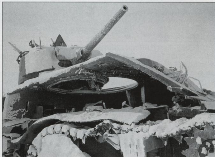
This close-up of the M4 to the left in one of the previous photos, tactical number 73, shows the results of a massive internal ammunition explosion that has peeled the right side armor back and blown the turret off the turret race.
