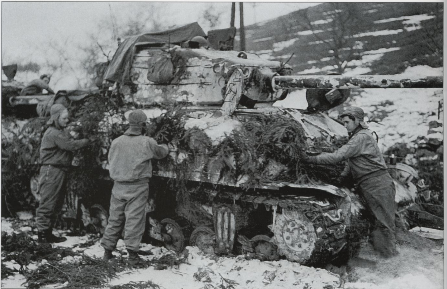
The crew of a M4A1 (76mm) of the 4th Armored Division add foliage to their tank in an effort to improve its camouflage near Kiewelbach, Luxembourg on 18 January 1945. This tank is fitted with metal chevron track and duck bill end extenders.
