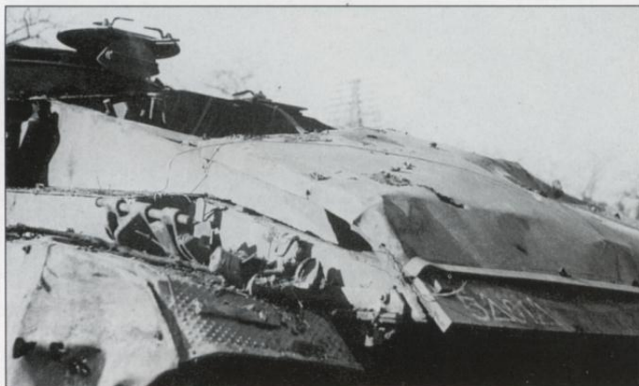
Besides the Panther tanks, five StuG III assault guns were converted for Panzer Brigade 150. Since they bore no resemblance at all to any US vehicle, their camouflage seems rather odd. The muzzle brake was removed, and side skirts added. This one was abandoned near the Baugnez crossroads, site of the infamous Malmédy massacre.
