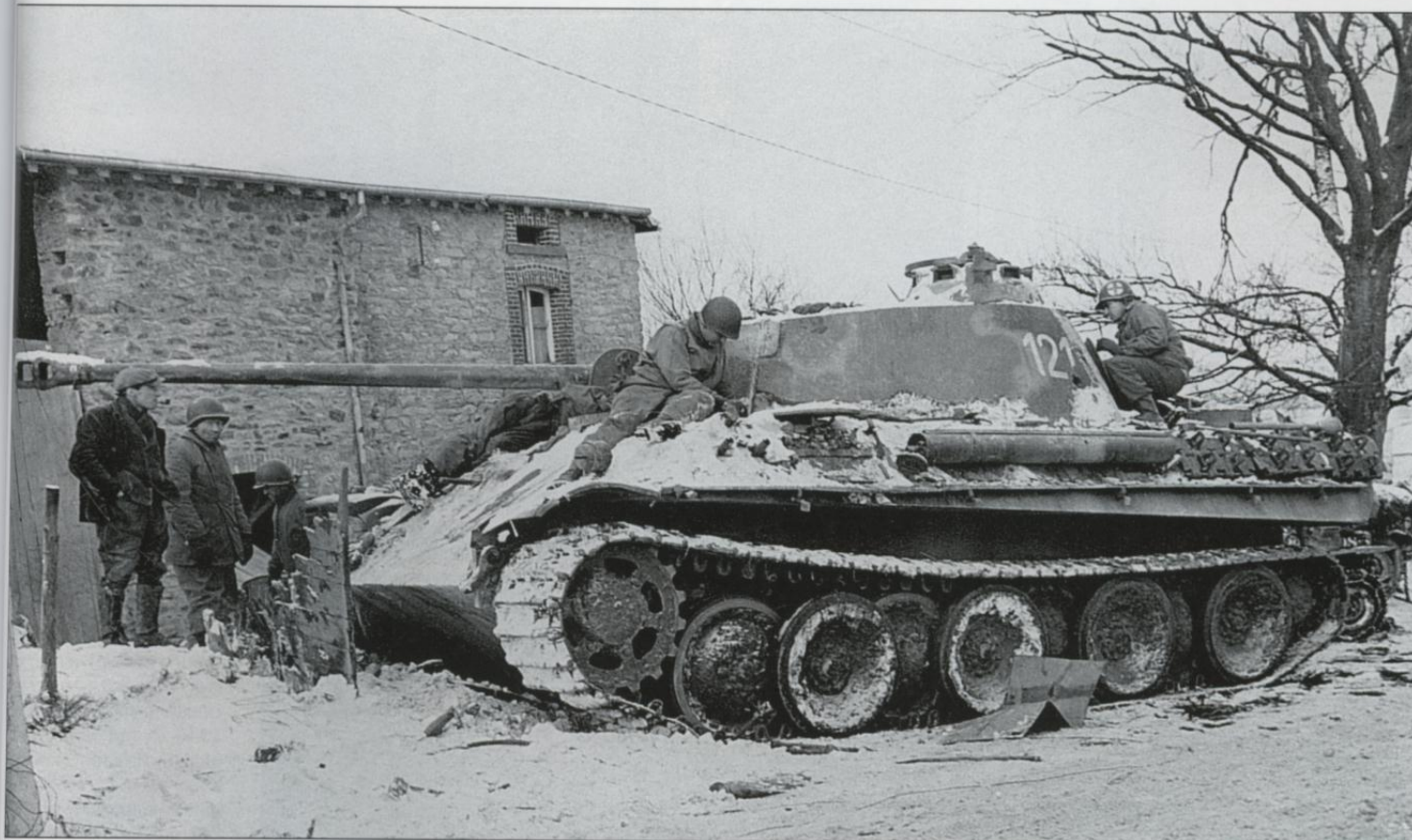
A Panther Ausf. G, tactical number 121 of the 9.Panzer Division, knocked out by a 57mm anti-tank gun during the fighting for Langlir, to the north-east of Houfallize, on 13 January 1945. Although the 57mm anti-tank gun was ineffective against the Panther's thick frontal armor, it could penetrate the side armor. Note the penetration in the turret side in the lower rear corner of the tactical number. The 9.Panzer Division typically painted its tactical numbers in plain white on the rear side of the turret.
