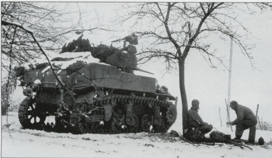
Tanks of the 2nd Armored Division support the 84th Division during the fighting near Amonines, Belgium on 2 January 1945. The lead tank appears to be a composite hull M4. It is fitted with the T54 metal chevron tracks with duck bill extenders. There was quite a bit of variation in the detail of the duck bills, as many were manufactured locally in shops in Belgium and France.
