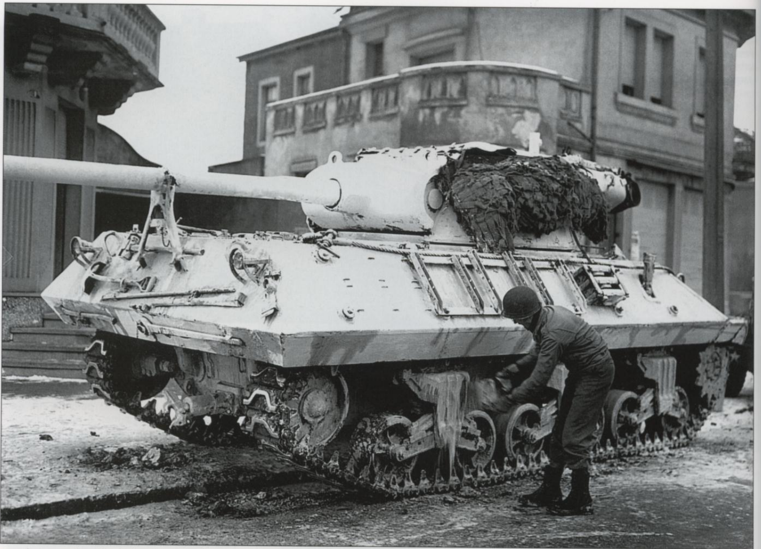
As snow closed in during the early winter of 1944-45, more and more US vehicles received a quick coat of whitewash like this M36 90mm GMC from one of the units of Patton's Third Army operating in Luxembourg in the final phase of the Battle of the Bulge on 3 January 1945. These paint jobs were often done in haste with mops, or in this case, with buckets.
