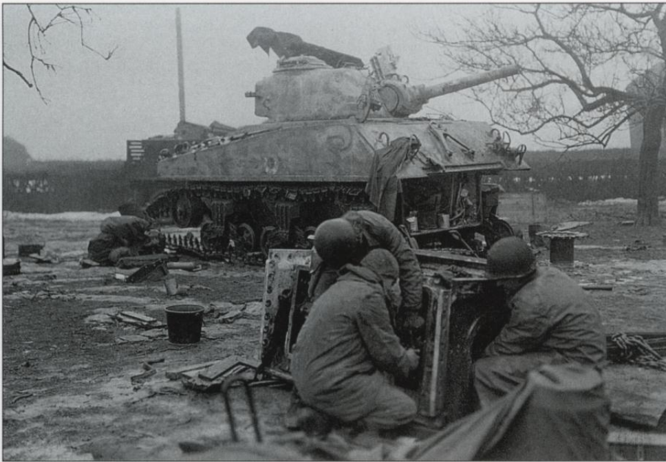
Following the heavy fighting in Belgium, the crew of a M4 (105mm) assault gun of the HQ Company, 69th Tank Battalion, 6th Armored Division, repair the transmission of their tank, tactical number 58, near Bastogne on 4 February 1945. (Patton Museum)
