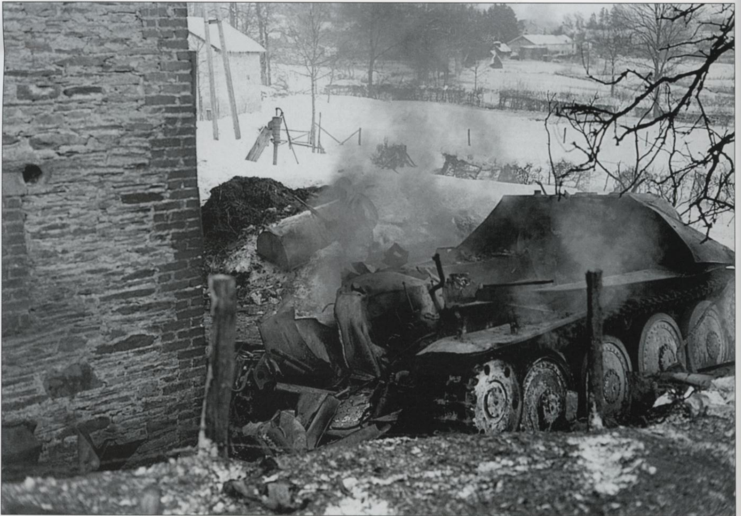
The following day, the 23rd AIB, 7th Armored Division moved out of St. Vith to capture the small town of Wallerode to the north east. This Jagdpanzer 38 (t) Hetzer was knocked out during the fighting. The Hetzer was widely used in Volksgrenadier divisions in lieu of the StuG III, but its thin side armor made it vulnerable as is so evident here. The combat photographer who photographed this scene was killed moments later during the fighting in Wallerode.
