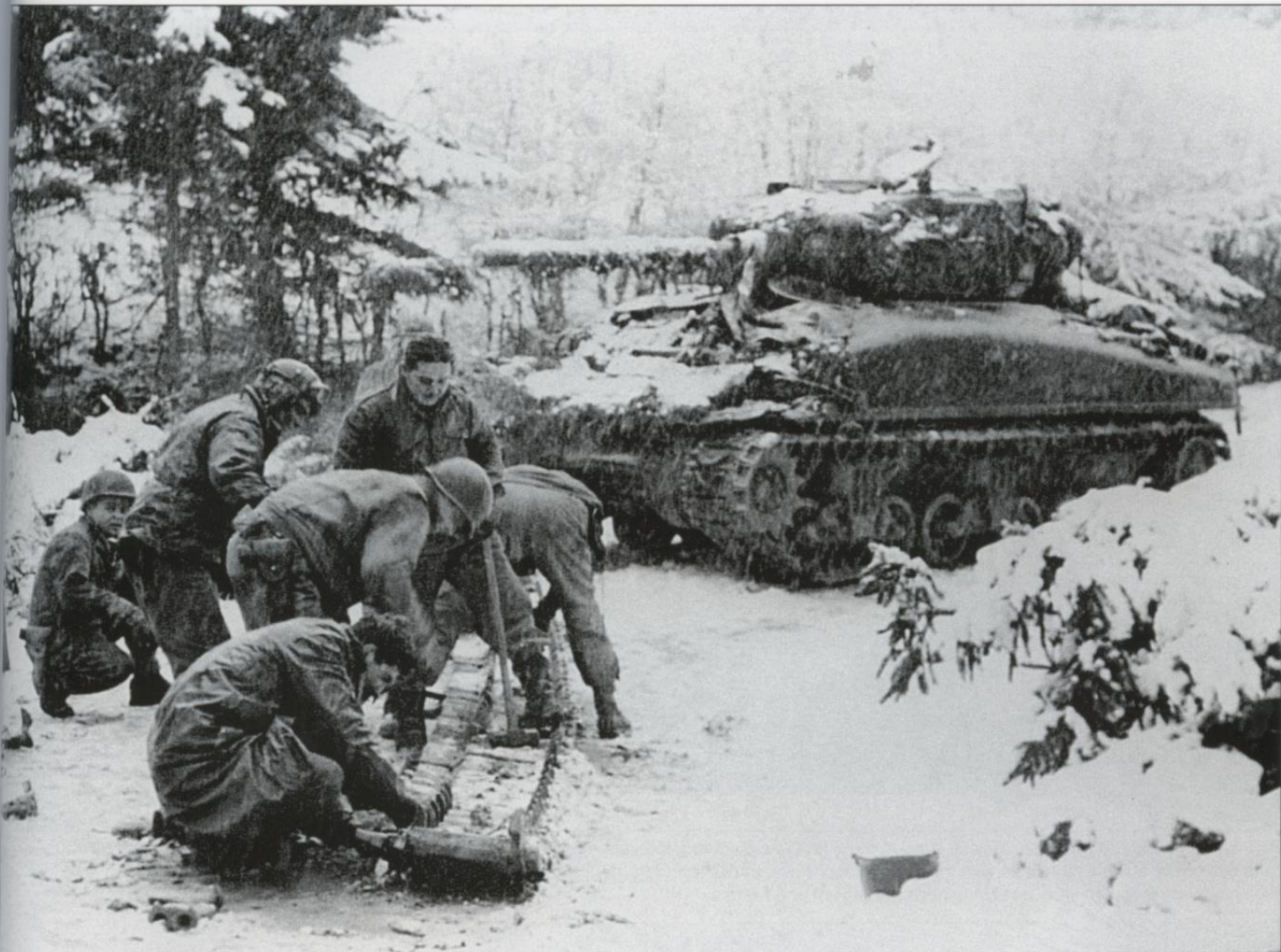
After the 2nd Armored Division blunted the German advance near Celles, it took part in the counter-offensive to reduce the Bulge. Here the crew of a M4A1 (76mm) medium tank repair the track in a wooded area near Amonines, Belgium in early January 1945 in the midst of a snow storm.
