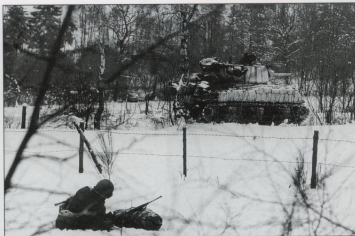
The 117th Infantry, 30th Division moved across the Ambleve along the Pont-Recht road on 17 January during the attack towards St. Vith. The 2/117th Infantry was supported by this M4A3E2 Jumbo assault tank, protected by sandbags along its side as well as its added armor.
