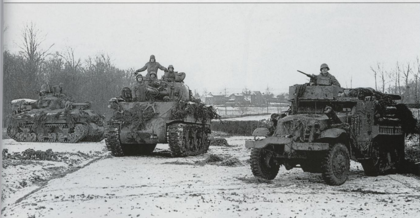
The HQ company of 2/32nd Armored Regiment, 3rd Armored Division move forward near Marche, Belgium on 31 December 1944. The tanks are M4 (105mm) assault guns, while to the right is a M3A1 half-track.
