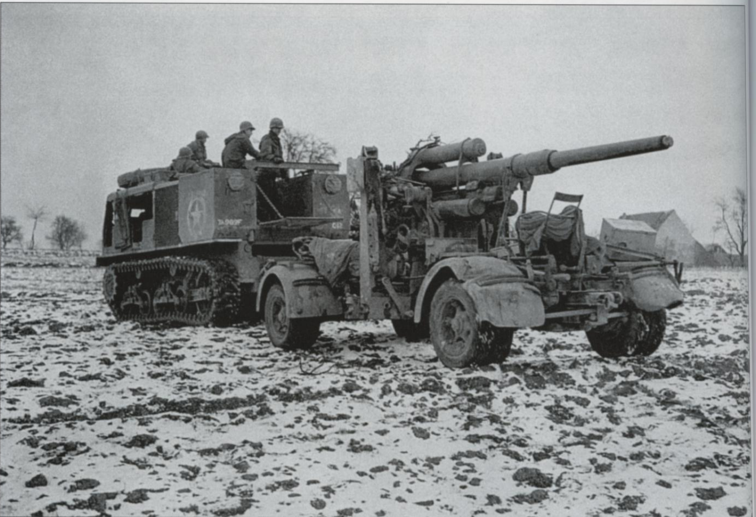
A M4 high speed tractor of Battery C, 989th Field Artillery Battalion recovers a German 88mm Flak 36 anti-aircraft gun on 5 January 1945. This unit operated 155mm guns in support of Patton's Third Army near Bastogne.
