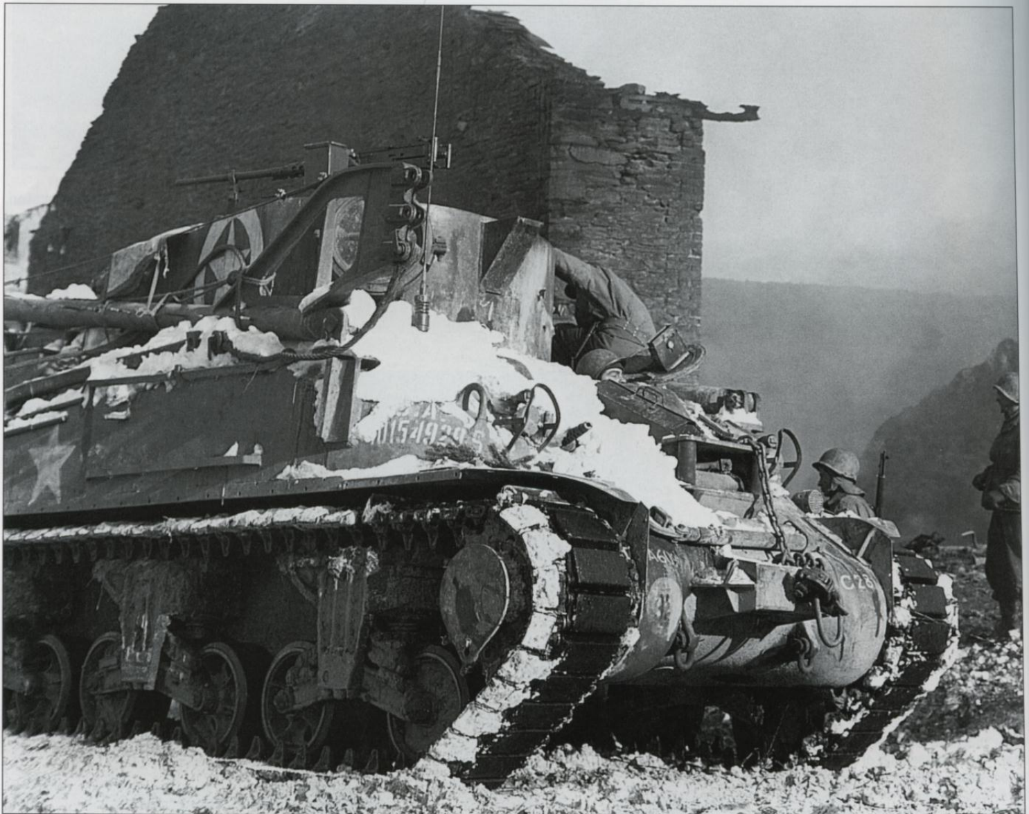
A M32B1 armored recovery vehicle of the 6th Armored Division moves to the outskirts of Bastogne on 14 January 1945 in anticipation of the push to break out of the pocket. The M32B1 was an armored recovery vehicle based on the hull of the M4A1 tank, fitted with a new turret, a winch, and an A-frame crane.
