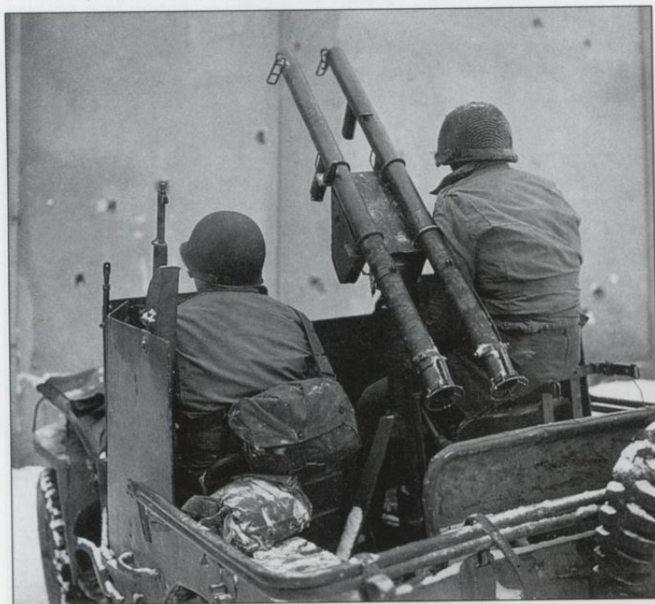
An intelligence and reconnaissance (I&R) platoon from the 60th Infantry, 9th Division developed this improvised mounting for a pair of 2.35 inch bazookas using the normal .50 cal heavy machine gun pedestal in a jeep. This vehicle was photographed in Belgium on 16 January 1945.
