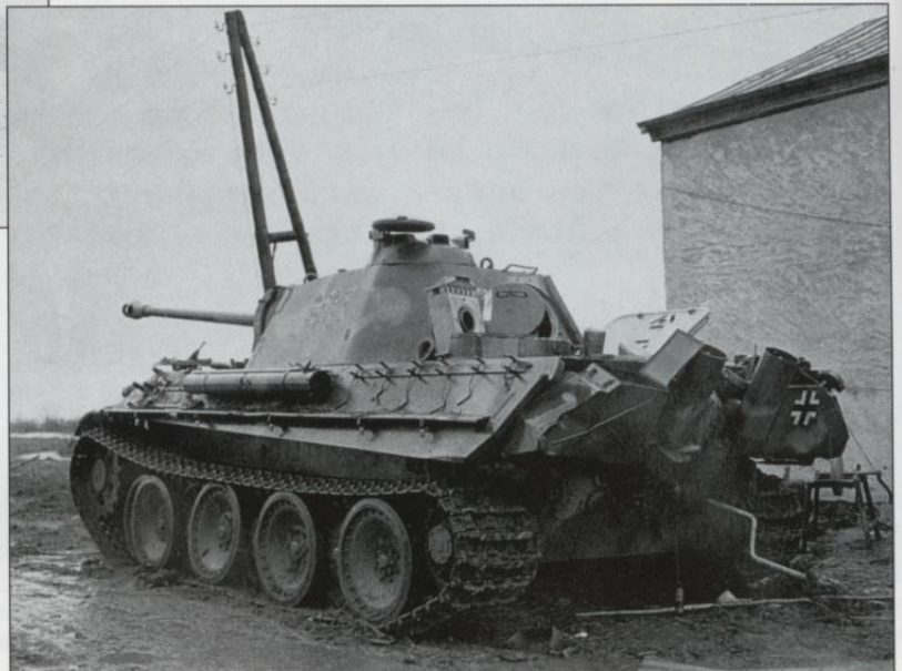
A Panther Ausf. G tank with the tactical number 301 from 2.Panzer Division abandoned near Clervaux, Luxembourg due to engine problems when the town was retaken by the 26th Infantry Division on 25 January 1945. Like most of the Panthers serving during the campaign, this is a fairly new vehicle, produced no earlier than October 1944 judging from the late style self-cleaning idler wheels. It also features the late flame dampers on the exhaust, and the crew compartment heater.
