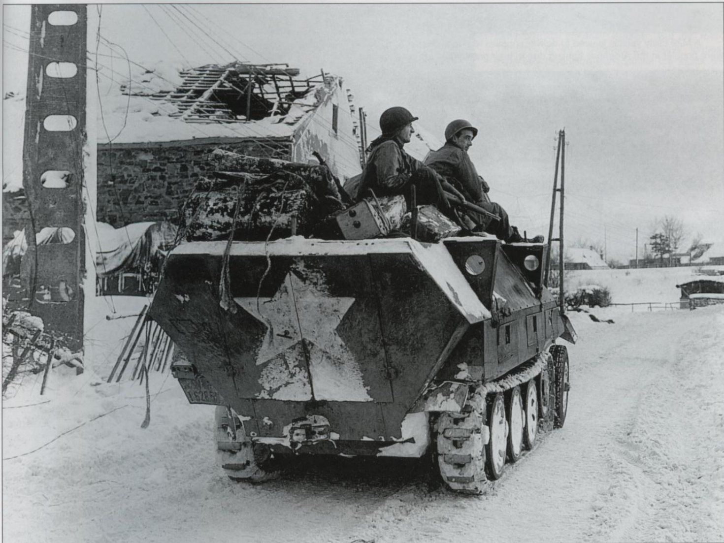
US units sometimes made use of captured German equipment. In this case, Co. L, 3/16th Infantry, 1st Infantry Division has adopted this SdKfz 251/7 combat engineer halftrack after prominently remarking it with white stars. It still carries its Wehrmacht license plate, and is being used to carry supplies near Schoppen, Belgium on 22 January 1945.
