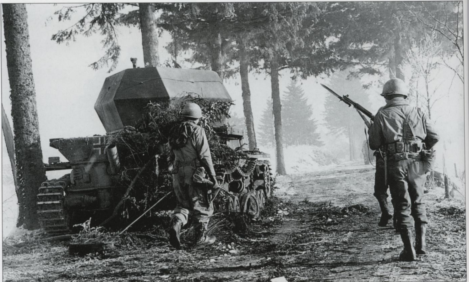
US infantry moves up north of Bastogne near Compogne, Belgium on 15 January past a disabled Flakpanzer IV Wirbelwind. This anti-aircraft version of the PzKpfw IV tank was armed with a four-barrel 20mm Flak 38 anti-aircraft cannon.
